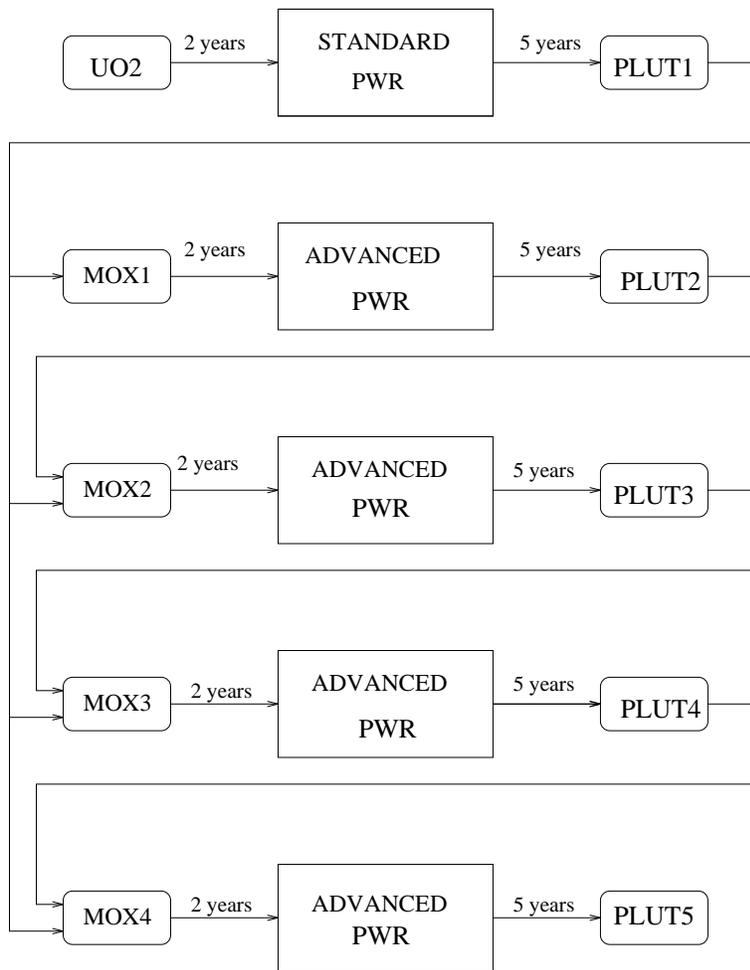
Figure 1: A schematic representation of the recycling calculations. The standard PWR has a MF ratio of two, the advanced PWRs all have MF ratios of 2, 2.5, 3, 3.5 or 4. A blending ratio of three has been used in the calculations, which means that each unloaded MOX assembly is mixed with three spent  $UO_2$  assemblies.
