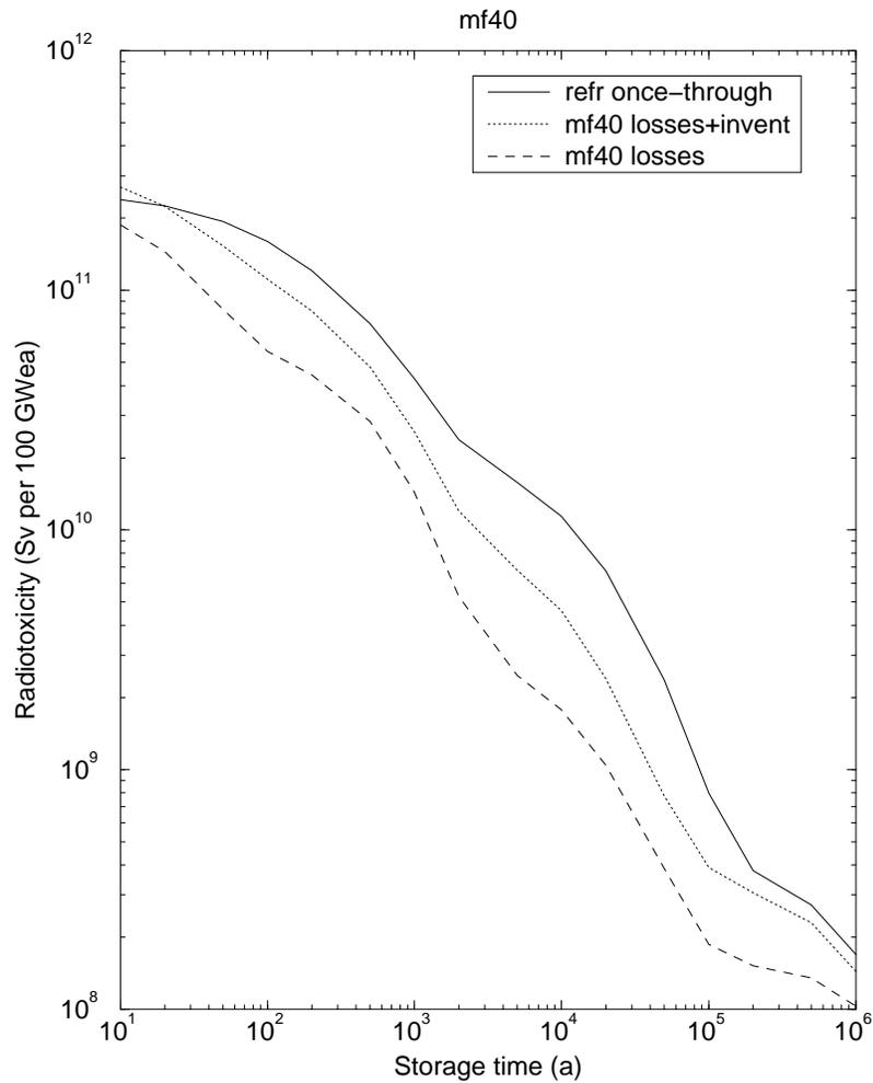
Figure 3: A comparison of the radiotoxicity of the reactorpark consisting of  $UO_2$  fueled reactors in once-through mode (refr), and of the reactorpark with plutonium recycling in MOX fueled reactors with  $MF=4$ . The plutonium after four times recycling is assumed to be disposed of (curve "losses+invent") or to be stored for further use (curve "losses").
