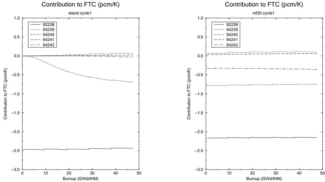
Figure 2: The contributions of the individual nuclides to the FTC for the  $UO_2$  fuel (left figure) and for the MOX fuel with  $MF=2$  as a function of burnup.
